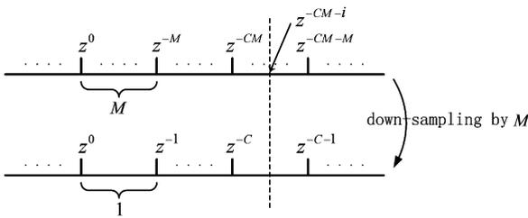
Fig. 3. Sampling of the low-pass channel in Fig. 1(c).
