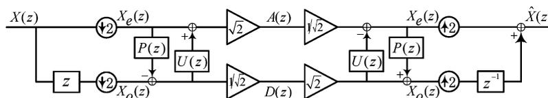
Fig. 6. Normalization of N–L-22 lifting wavelet.
