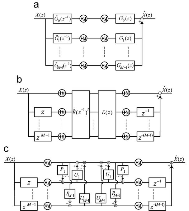
Fig. 1. Three representations of wavelet filter bank: (a) channel representation, (b) polyphase representation and (c) lifting representation.
