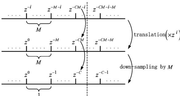
Fig. 4. Transaction and sampling of the  $i$ th high-pass channel in Fig. 1(c).
